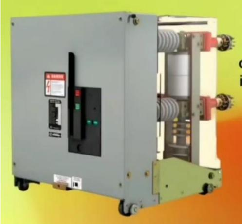
VCB stands for Vacuum Circuit Breaker. In vacuum circuit breakers, the vacuum is used as the arc quenching medium Vacuum offers the highest insulating strength. So it has far superior arc quenching properties than any other medium (oil in oil CB, SF6 in SF6 circuit breaker).
